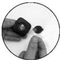
3.take out the insulation sheet
