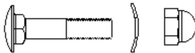
Bolt M10 x 56 (4 pcs) Arc washer \Phi 10 \times \Phi 20 \times 1,5 (4 pcs) Domed nut M10 (4 pcs)
