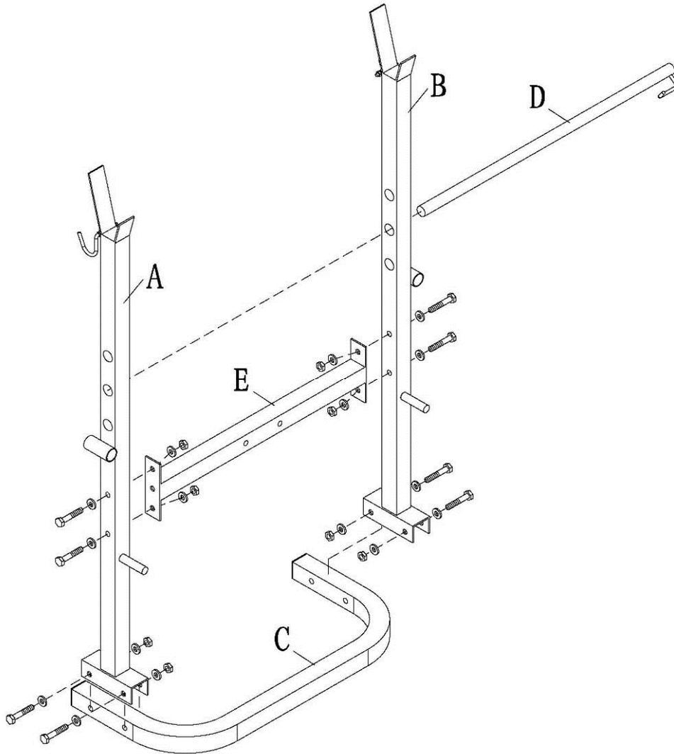
Securely fasten each upright beam (A、 B) to the bottom beam (C) use the M10\*60 bolts as shown. Then fasten the cross beam (E) to each upright beam (A、 B) use the M10\*60 bolts.
