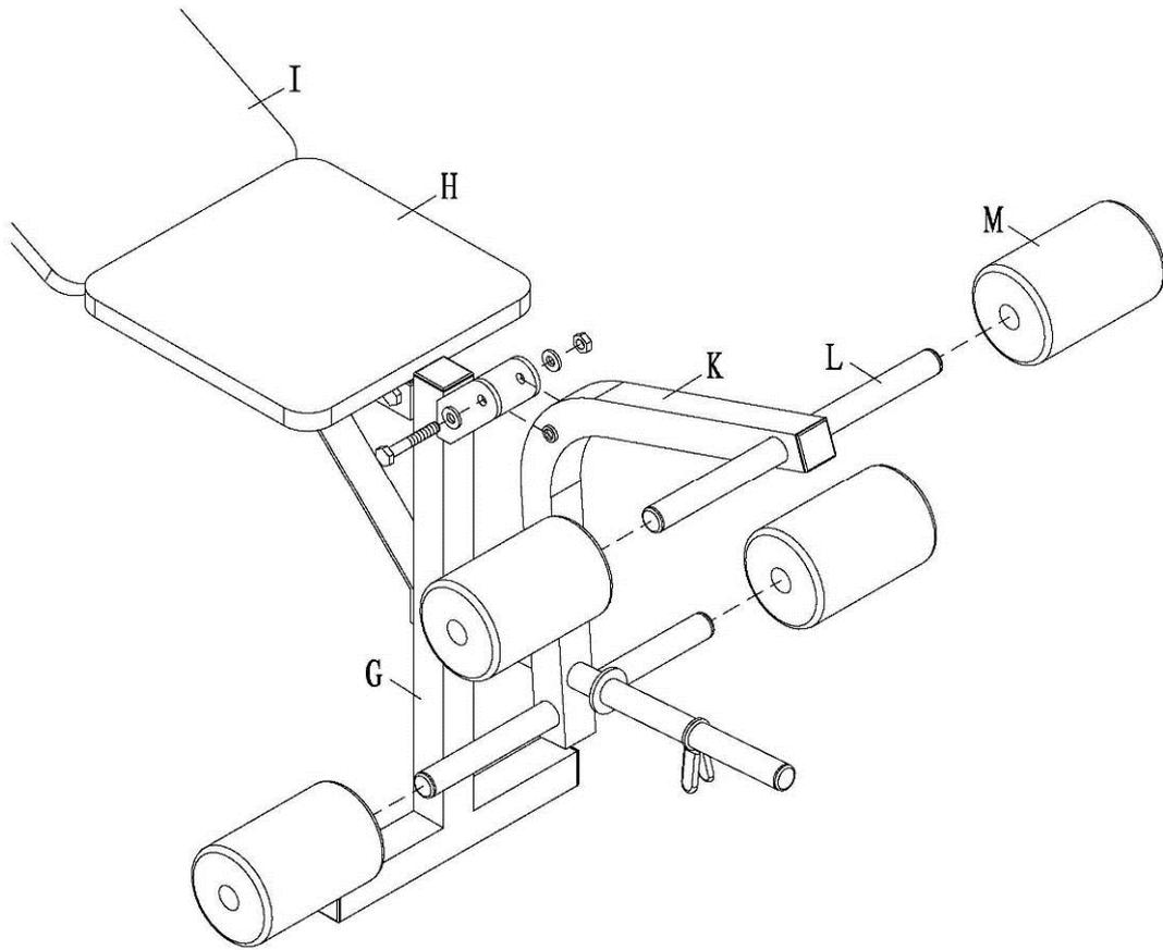
Securely fasten the leg extension beam (K) to the front beam (G) using the M10\*65 bolt as shown. The leg extension should be tightened so that it will move when you pull on it without weights and stay in that position, but not so tight because that will be difficult to move.
