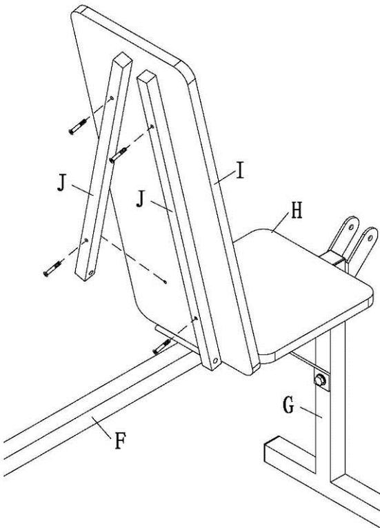
Attach the two square metal bench seat supports (J) to main frame (F).
