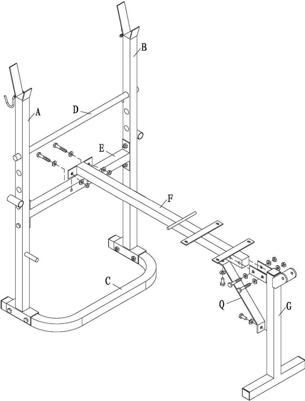
Securely fasten the main beam(F) to the cross beam(E) use the M10\*60 bolts as shown.
