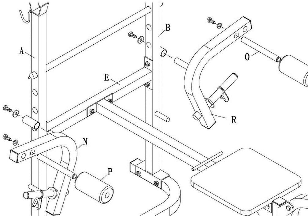
Fasten each butterfly arm (N&R) on each of the uprights as shown using the M10\*25 bolts. The bolt should be put through the nylon inserts in the upright first and then the butterfly arms assembled and tightened.
